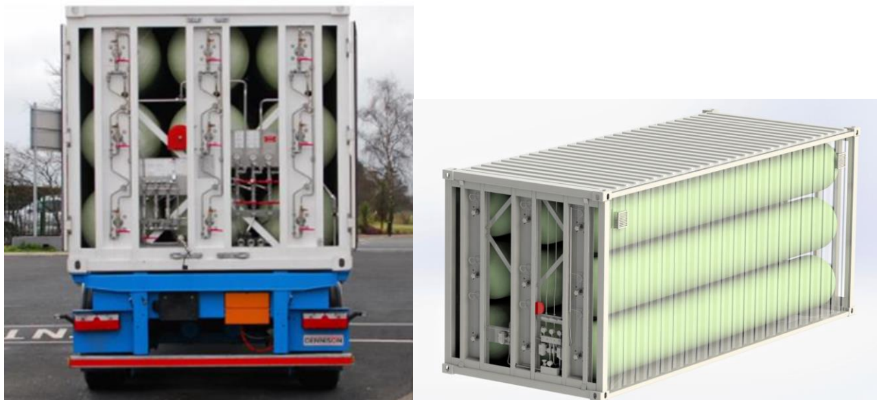
Figur 2: Konteinerbasert gassflak (ref. www.uac.no )
